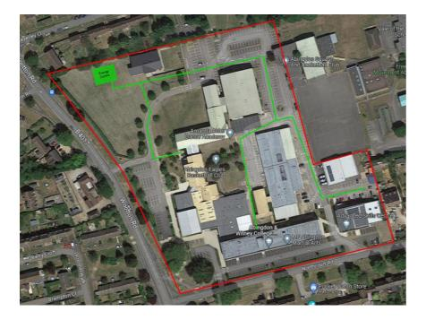
The campus layout enables a clear route to distribute low temperature hot water pipework to the individual building plant rooms, where substations could be located. Installing substations within each building creates hydronic separation between the buildings and the heat network, enabling ease of phased building connection and isolation for maintenance.
